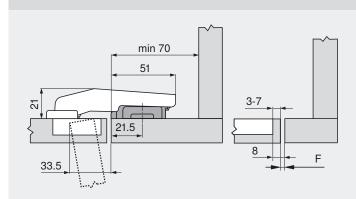
Move standard mounting plate fixing positions 15.5 mm nearer the edge of the blind corner (i.e. set back by 21.5 mm).
