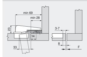
Fixing position from inside edge of muntin: 14 mm Special mounting plate for blind corner application: 199.8130
