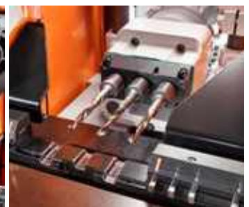
Horizontal drilling (only possible with MINIPRESS top)
