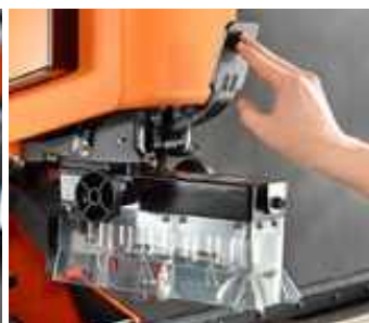
Tool-free assembly of drilling heads
