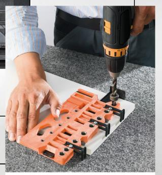
The Universal drilling template offers flexible marking and pre-drilling for front fixings including gallery, drawer back, drawer base and AVENTOS front fixings. You can calibrate the jig to ensure you don't drill the holes too deep and damage the drawer front.
